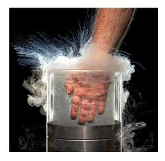
3. Fog clouds do not define the vapor cloud: They define the area where the vapours are still cold enough to condense the moisture in the air. The vapours can extend well beyond the fog cloud, depending on the product and atmospheric conditions. Although fog clouds may be indicative of a release, they must never be used to define the leak area and should not be entered by anyone. The dense fog clouds associated with the handling or transfer of cryogenic liquids can obstruct visibility.
